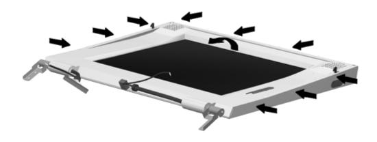
Figure 5-32. Removing the Display Bezel
